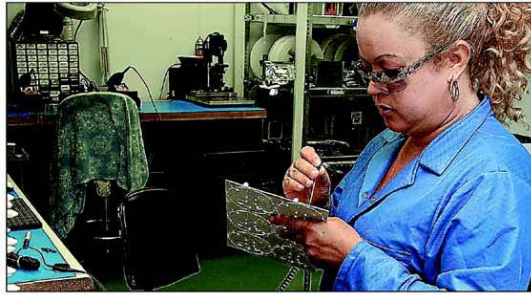
Lydia Santos, of New London, tests the microprocessor boards that will eventually end up in a military vehicle at the Thomas G. Faria Corp. plant in Uncasville. The plant makes instrumentation for the auto industry. Adena Stevens / The Day
